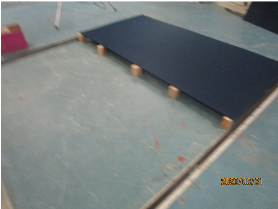
Figure 2 – Specimen partially installed, spacer array
